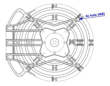
900 mm / 3 ft older model:Mounting needs longer screws and12 mm long distance tubes
